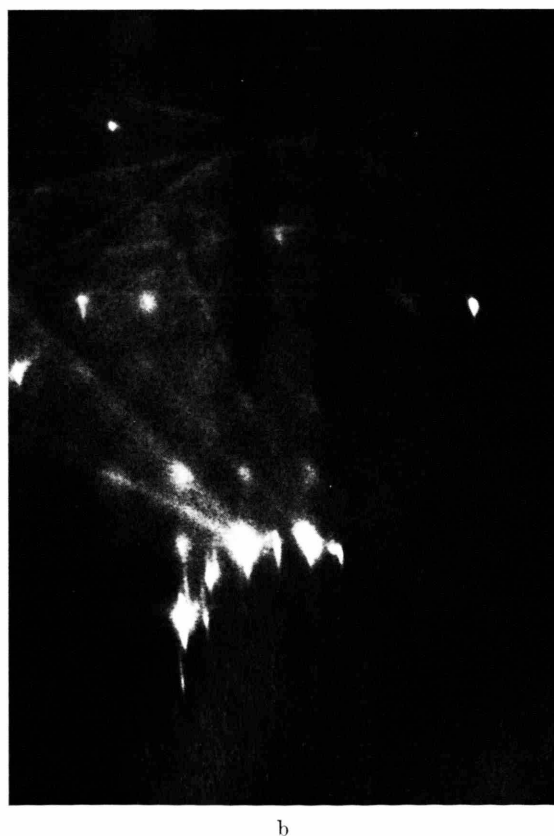
Fig. 2. RHEED diagram from Ag ( \approx 018)-Cl. Primary beam nearly parallel to Ag [010]. +: Ag streaks. o: additional streaks from Ag (001) c ( 2 \times 2 )-Cl.
